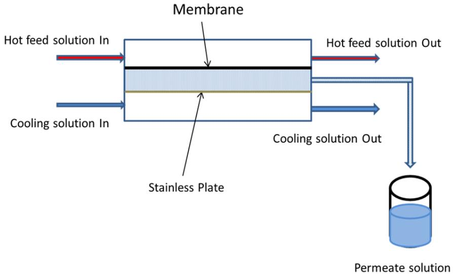
Figure 1. Schematic representation of the MD module
