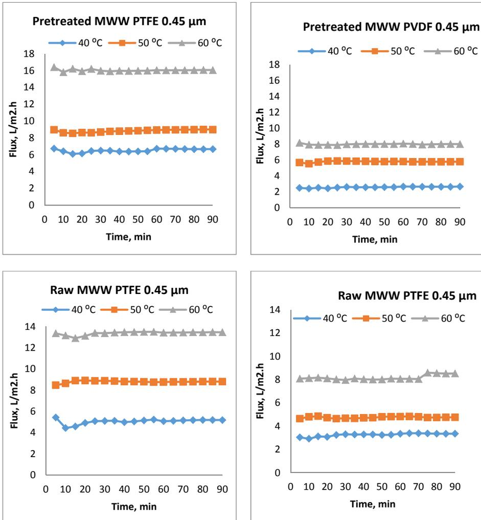
**Figure 4.** The TMF behavior with raw and pretreated MWW at different feed temperature with PTFE and PVDF membranes
