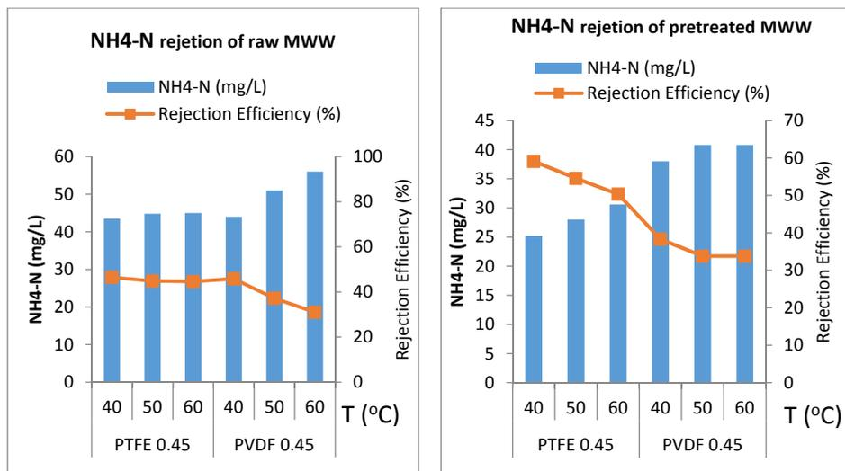
**Figure 3.** NH<sub>4</sub>-N content of the MD permeate solution and the rejection efficiency with raw and pretreated MWW
