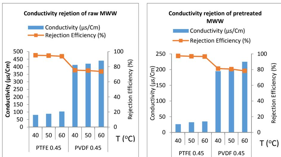
Figure 2. The conductivity of the MD permeate solution and the rejection efficiency with raw and pretreated MWW
