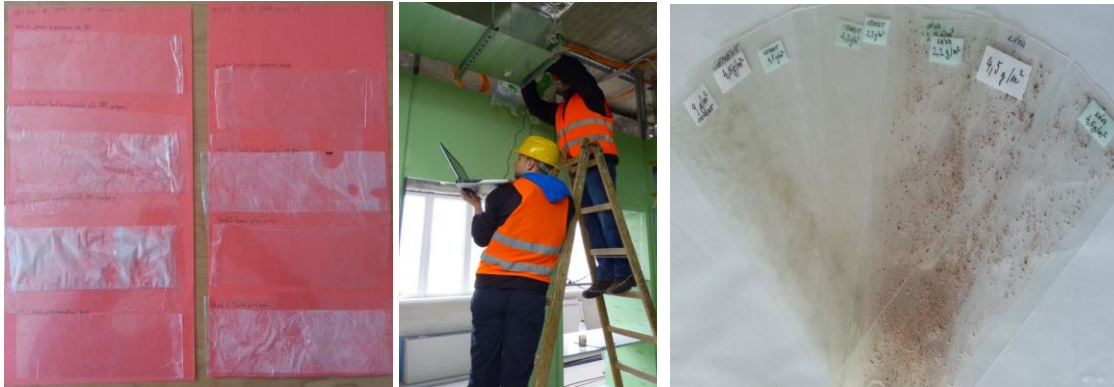
Figure 5. Example of assessment of pipework contamination by visual inspection using checking benchmark method (right), the samples (left)
