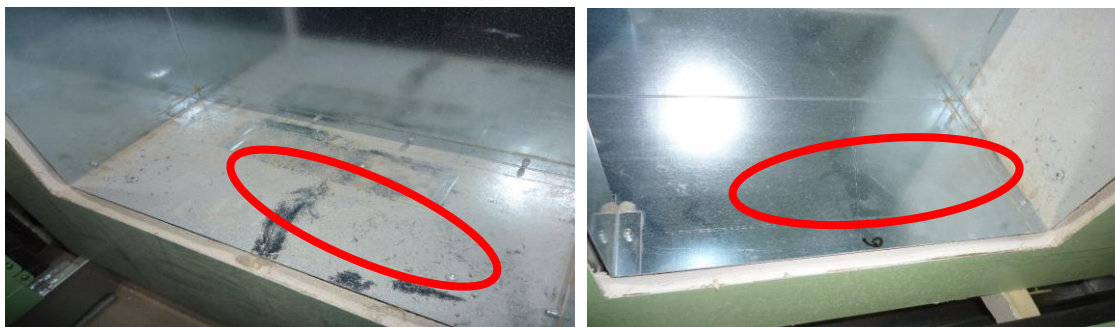
Figure 4. Demonstration of sampling by using tape for comparison with a standard dust concentration
