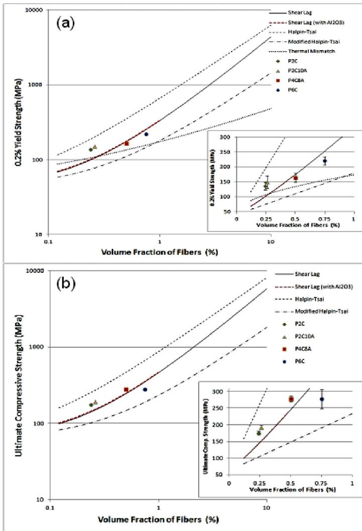
**Figure 3.** Comparison of experimental and calculated data of CNT /Al composites (a) Predicted 0.2% yield strength – volume fraction (b) predicted ultimate compressive strength – volume fraction of carbon nanotube curves calculated with different models.
