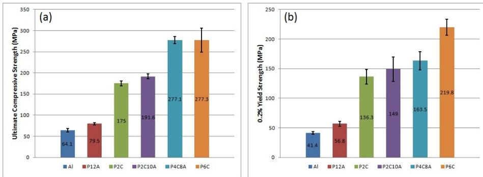
Figure 2. D. Comparison of average (a) ultimate compressive strength (b) 0.2% yield strength
