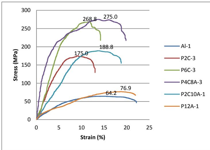
Figure 1. C. Typical stress-strain curves of matrix material and different type of composite materials (ultimate compressive strength values are written on curves)
